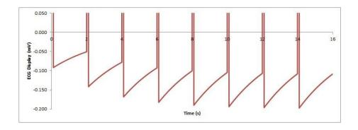
A pulse train of 3mV/100ms impulses repeated at 0.5Hz (30bpm), expanded to see the effect around the baseline. The slope of the last pulse is clearly different to the slope of the first pulse
