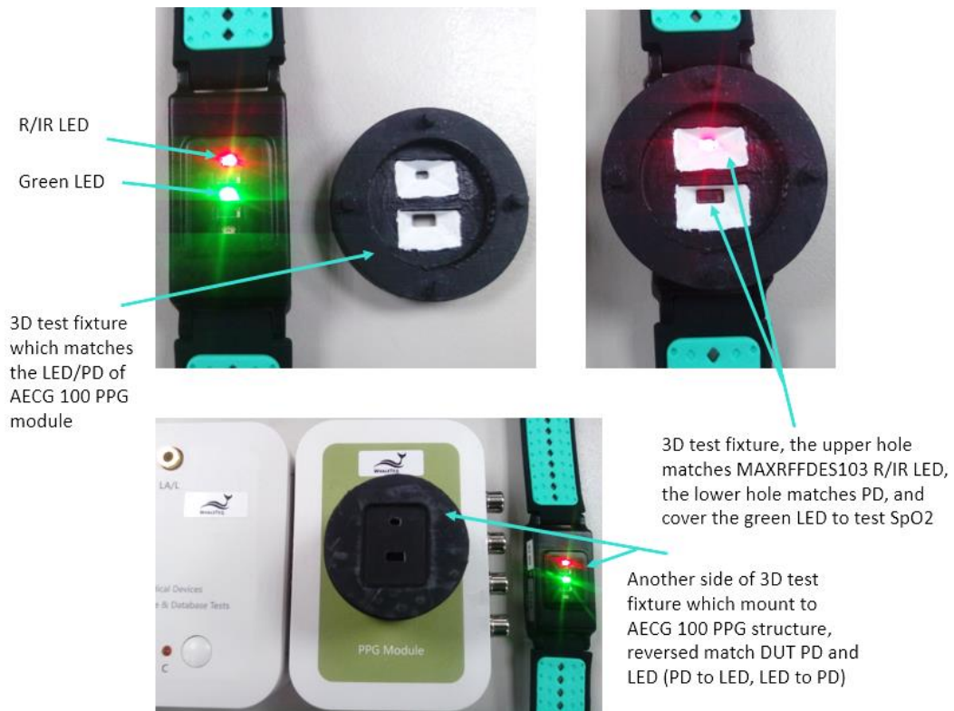
Fig. 2 The 3D-printing fixture is tightly fastened onto AECG 100 PPG fixture base
