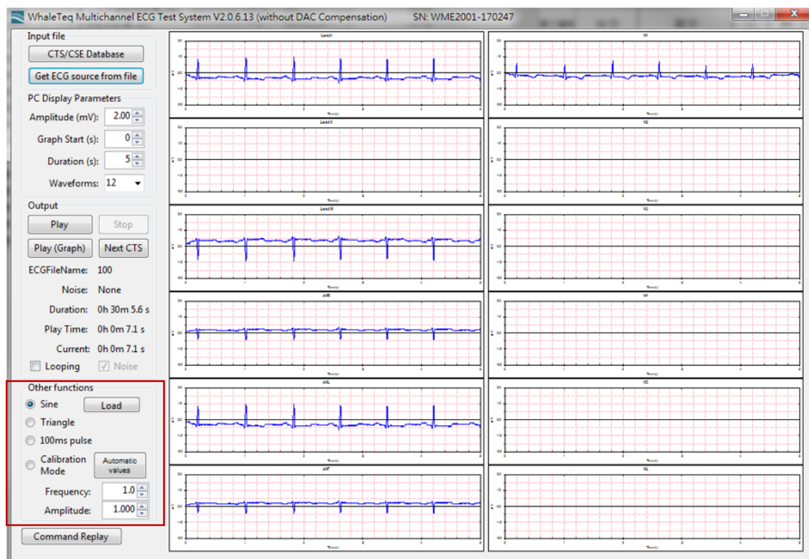
Figure 7. MECG 2.0 outputs MIT 100 data and changes the lead mapping. The right half shows the waveform of each lead that should be displayed on the EUT ECG
