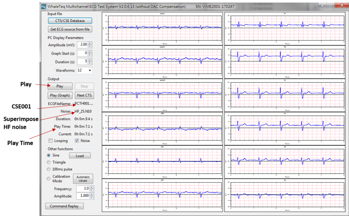
Figure 5. An example of the MCEG 2.0 selecting the CSE001 data output and superimposing high-frequency noise. The right half displays the waveform that each lead on the EUT ECG should show.
