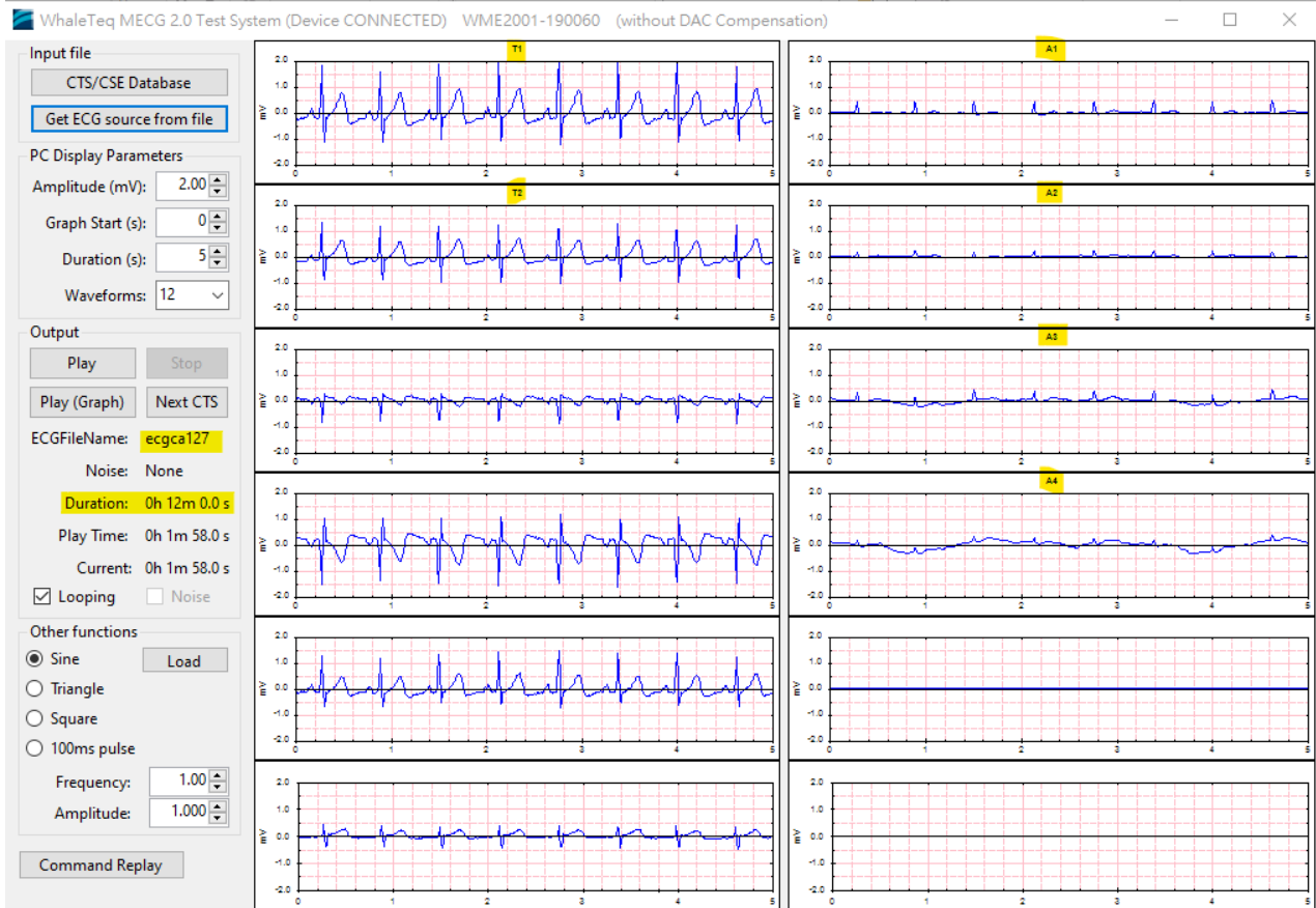
Figure 6: Display T1/T2/A1~A4 output waveform in the main screen of MEGC software
