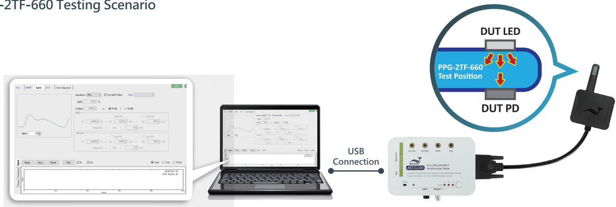
(The image illustrates the testing scenario of the PPG-2TF-660 and AECG100. Please refer to the user manual for detailed installation and instructions when using PPG-2TF-660 with AECG100 or SECG 5.0 AIO.)
