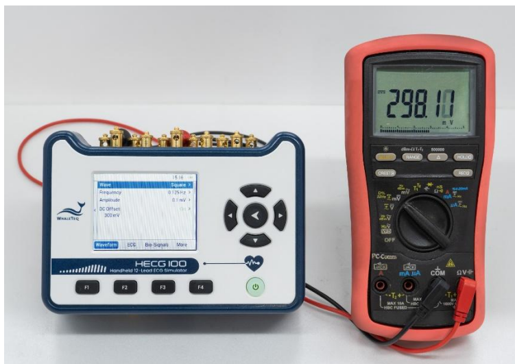
Figure 63: Self-calibration Setup for DC Voltage Verification
