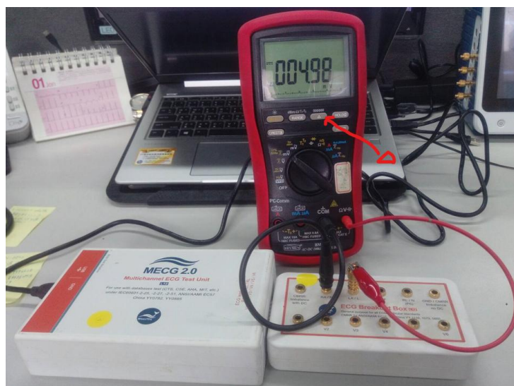
Figure 12: Connection to a multimeter
