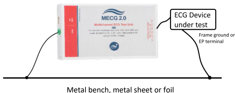
Figure 3: Set up a noise-free test environment
