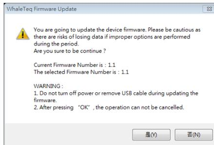
**Figure 44: Manually Update Firmware (Step 4)**
