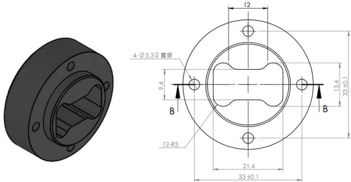
Figure 6: Mechanical Drawing of Bottom LED Holder
