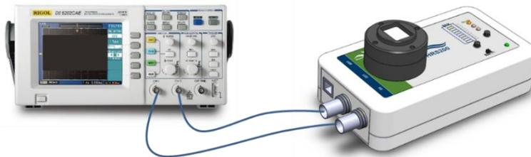
Figure 12: Cabling Diagram of Connecting the HRS200 to an Oscilloscope
