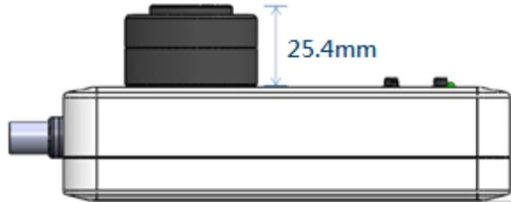
Figure 9: Height of Fixture Mounting Base
