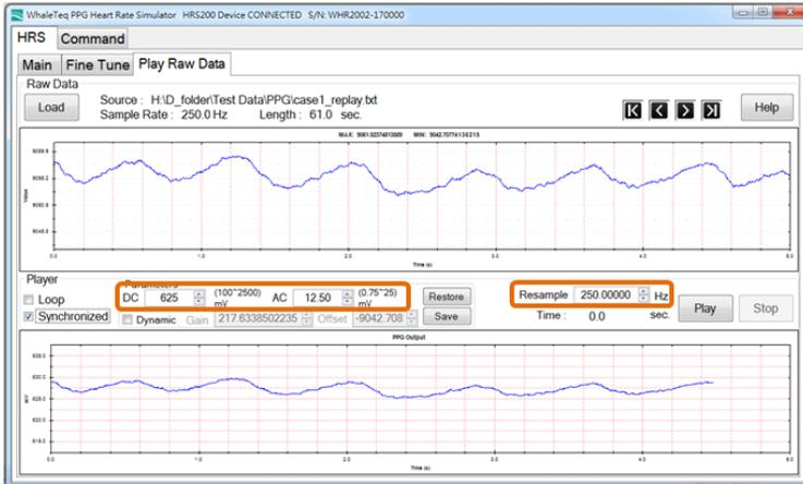
Figure 33: Play Recorded Raw Data Waveform with Normal Range Signal (Step 3)
