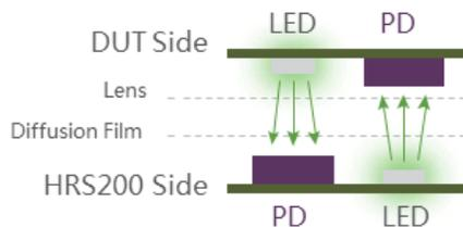
Figure 2: The Interaction Between HRS200 and DUT
