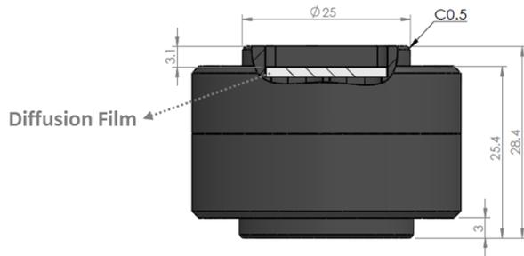
Figure 7: Sectional View of Fixture Mounting Base
