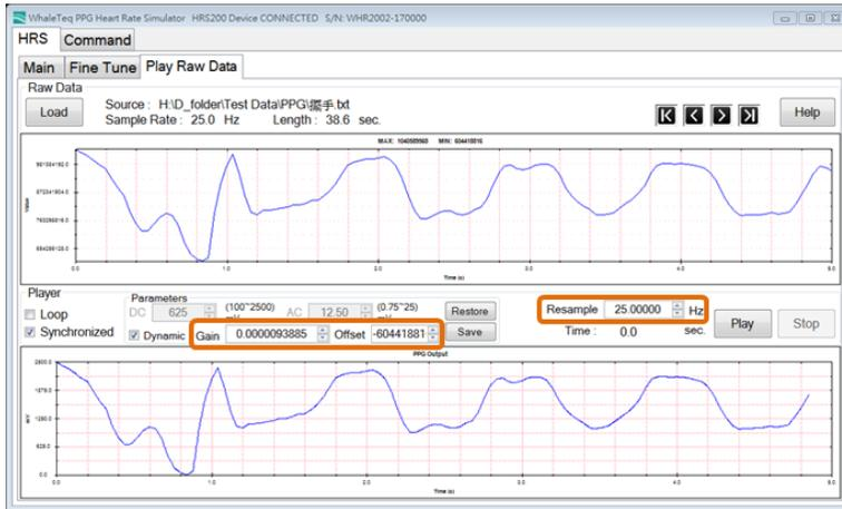
Figure 38: Play Recorded Raw Data Waveform with Dynamic Range Signal (Step 4)
