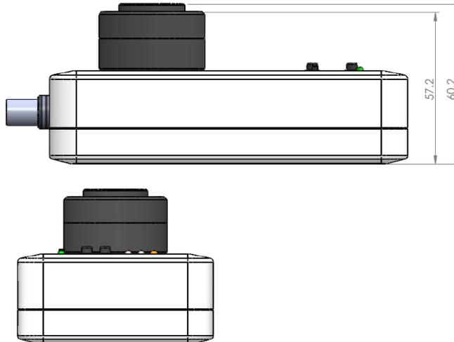
Figure 10: Height of Fixture Mounting Base and HRS200
