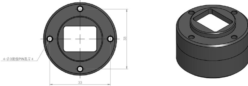
Figure 4: Mechanical Drawing of Fixture Mounting Base
