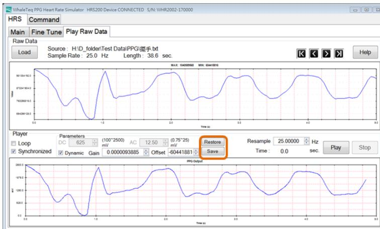
Figure 39: Play Recorded Raw Data Waveform with Dynamic Range Signal (Step 5)
