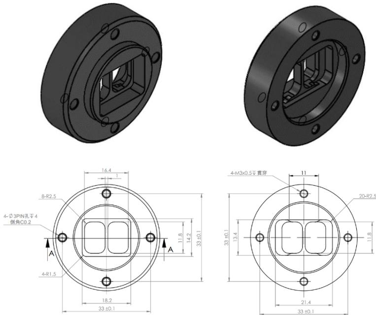
Figure 5: Mechanical Drawing of Top LED Holder
