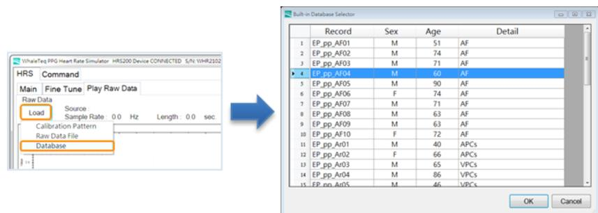
Figure 28: Activate HRS200 Full Database Set (Step 1)
