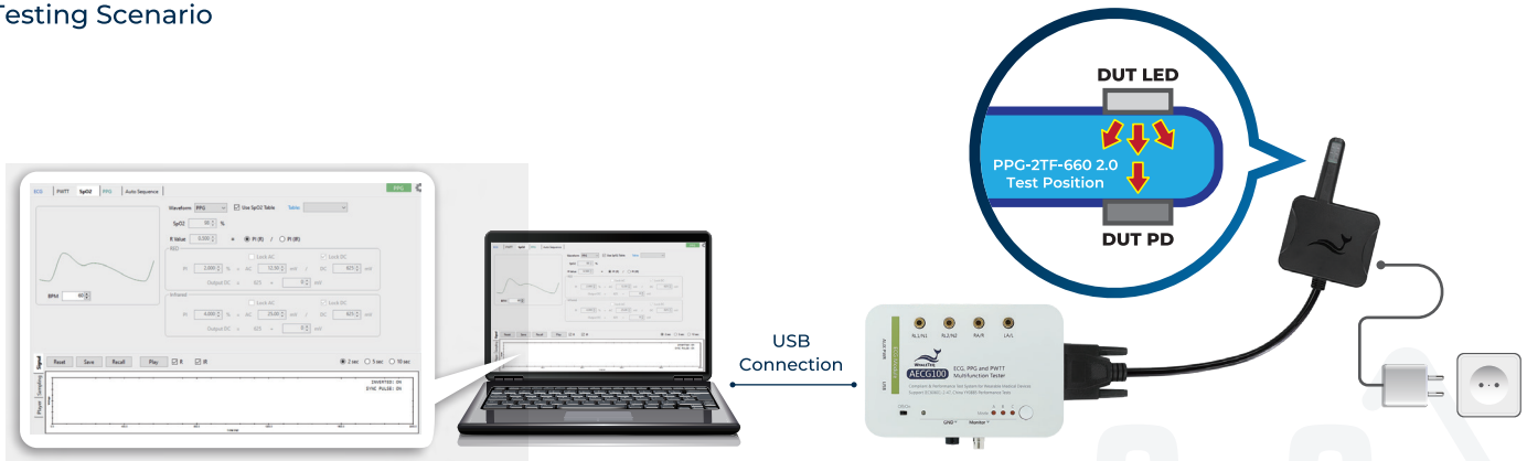
(The image illustrates the testing scenario of the PPG-2TF-660 2.0 and AEGC100. Please refer to the user manual for detailed installation and instructions when using PPG-2TF-660 2.0 with AEGC100 or SECG 5.0 AIO.)
