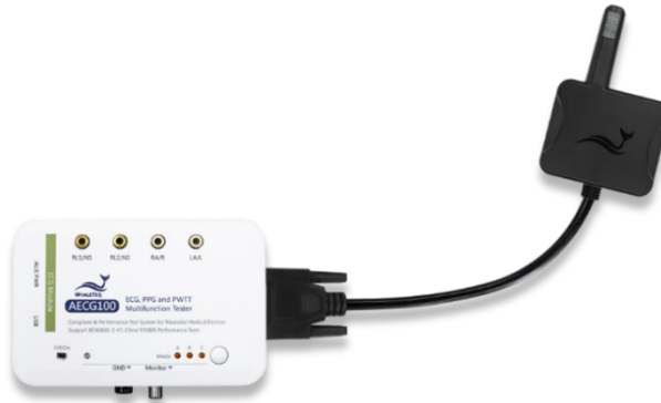
Figure 6: Direct Connection between AECG100 and PPG-2TF-660
