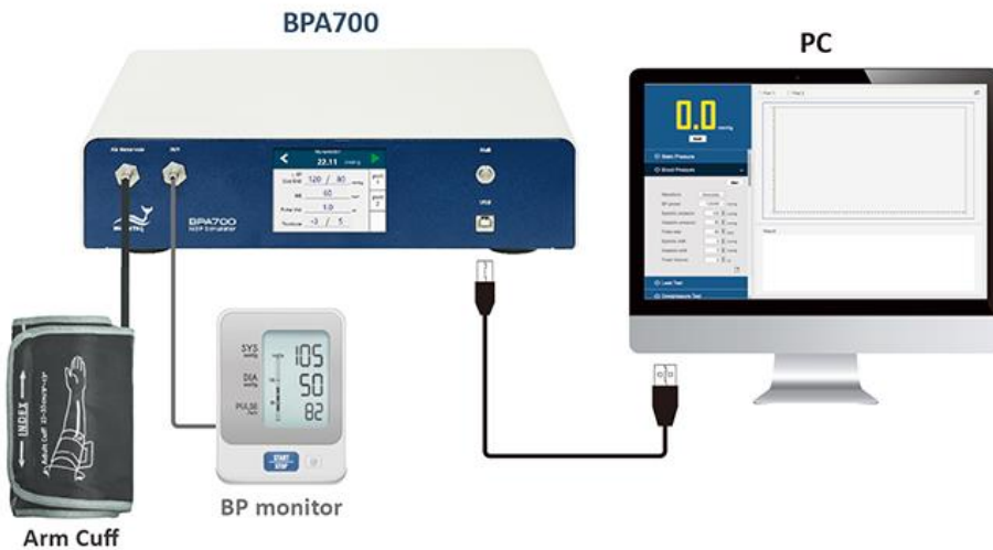
Figure 5: The Configuration of Arm BP Monitor
